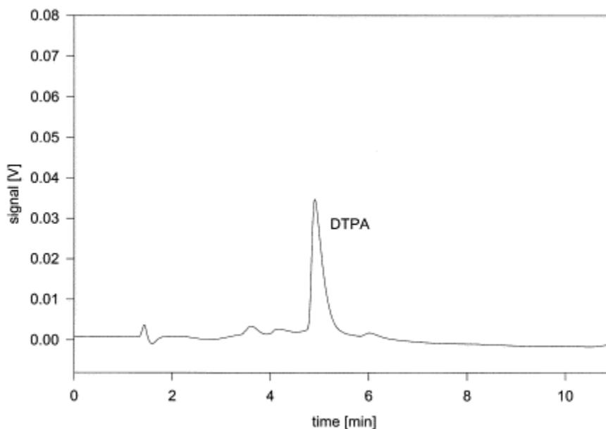
**Figure 2:** A typical DTPA chromatogram at a concentration of  $200\text{mg l}^{-1}$  DTPA [10]
